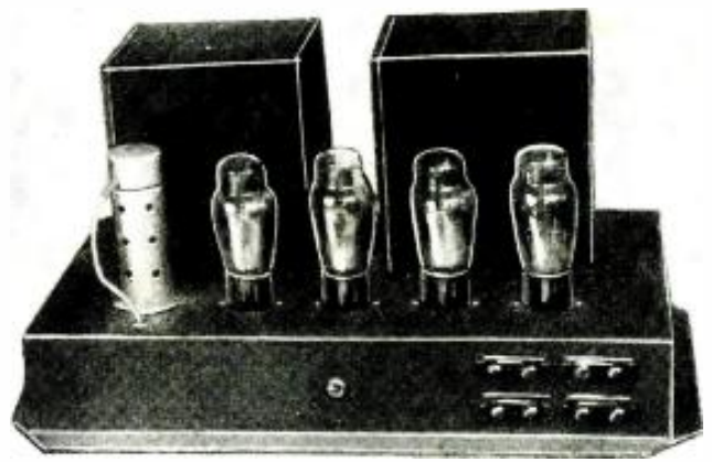
Fig. C, left; Fig. D, above. A 10 W., direct-coupled power amplifier with nearly flat response (left). A 28 W., direct-coupled power amplifier having fine output quality (above).
